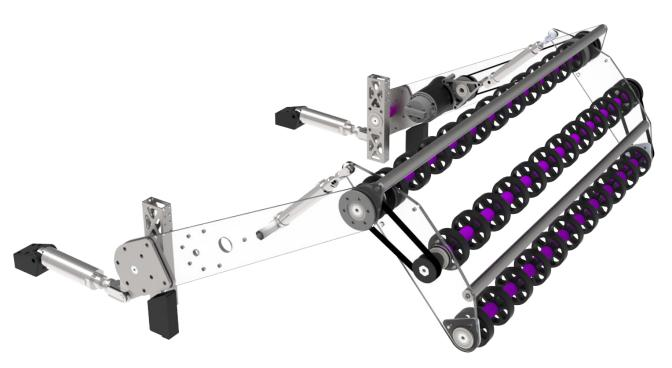
Double actuated intake designed to withstand high impacts and abuse during play.
