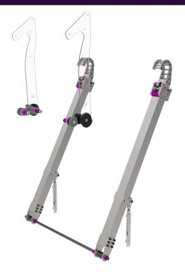
Two sets of 2 stage telescopic arms, and a pair of static hooks allow us to traverse the rungs.
