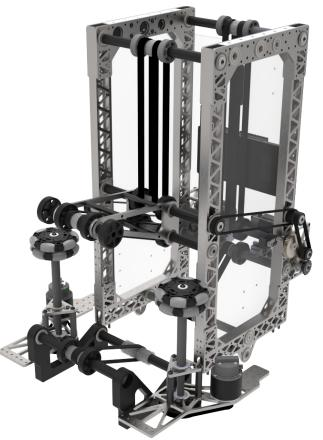
Two subsystems control the cargo in the robot, the conveyor and the feeder. Using an IR color sensor we are able to maintain an even pace of shooting and collecting.
