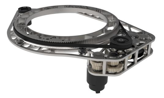
The turret allows the robot to quickly score cargo from any orientation and location on the field. It is powered by a Falcon-500 motor, and controlled by an absolute encoder.
