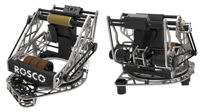
The shooter contains dual-flywheels with an adjustable hood angle to enable shooting from every location on the field. A Limelight camera vision tracks retro-reflective tape on the high goal to aim the turret, control the hood angle, and adjust the flywheel speed to ensure a successful shot.
