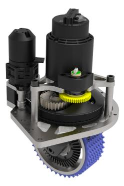
The drivetrain allows the robot to maneuver around the field quickly and precisely. This year's design is a custom swerve drivetrain that we developed over the past few years.
