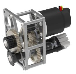
The Conveyor gearbox provides the power to the Conveyor, the Feeder and the Climb in the endgame. There are two similar gearboxes that attach to each side of the conveyor structure, one controls the conveyor, and the other one controls the feeder. In the last seconds of the match, both of the gearboxes combine using a dog shifter, in order to power the climber's telescopic arms.
